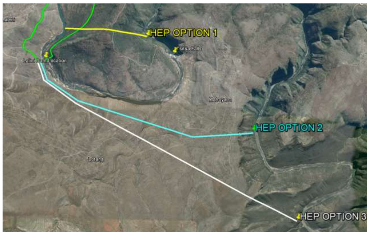
Figure 12-6: Hydropower Water Transfer Conduit Options
